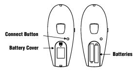
2 Insert the supplied batteries, making sure that the positive (+) and negative (-) ends of each battery match the polarity indicators inside the battery housing.
